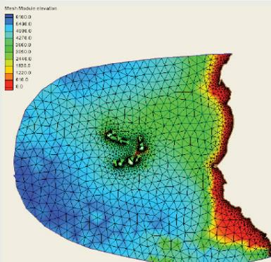
Figures 3.1 The ADCIRC storm surge model was installed and run for the Cape Verde islands; the model catchment was quite large (Figure 3.1).
