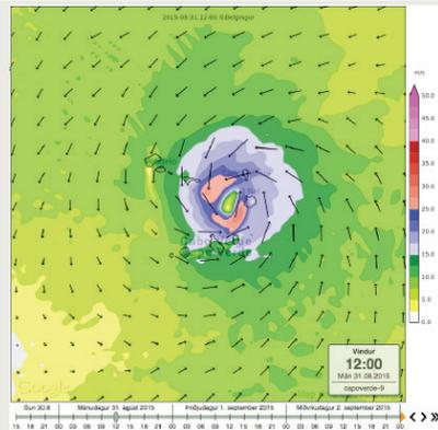
Figure 2.2 captures the same area 24 hours before the storm; the hurricane's centre and simulated winds are in close agreement with observations.
