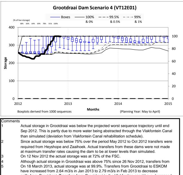
spills from Grootdraai. Transfers from Grootdraai to the Vlakfontien canal have decreased from 2.76 m3/s in Jan 2013 to 0.127 m3/s in Feb 2013 which is below the monthly target of 1.07 m3/s
